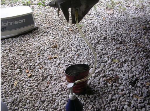
Notice how in the above picture how they are 2 phillips screws you can undo.....the screw on the right holds the gears for the propeller in place....DON'T LOOSEN THAT SCREW!!!!
