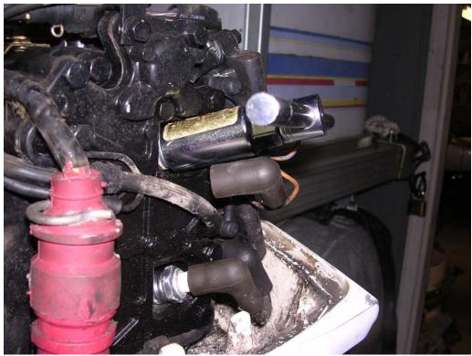
When spraying the fogging oil....DO NOT LOOSE THE RED SPRAY TUBE IN THE CYLINDER!!!...you will have a new problem otherwise!
